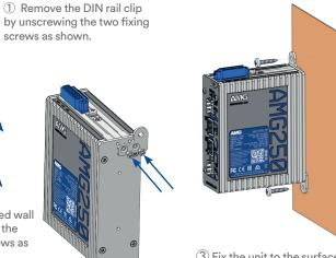
③ Fix the unit to the surface using two appropriate screws (screws not provided)
